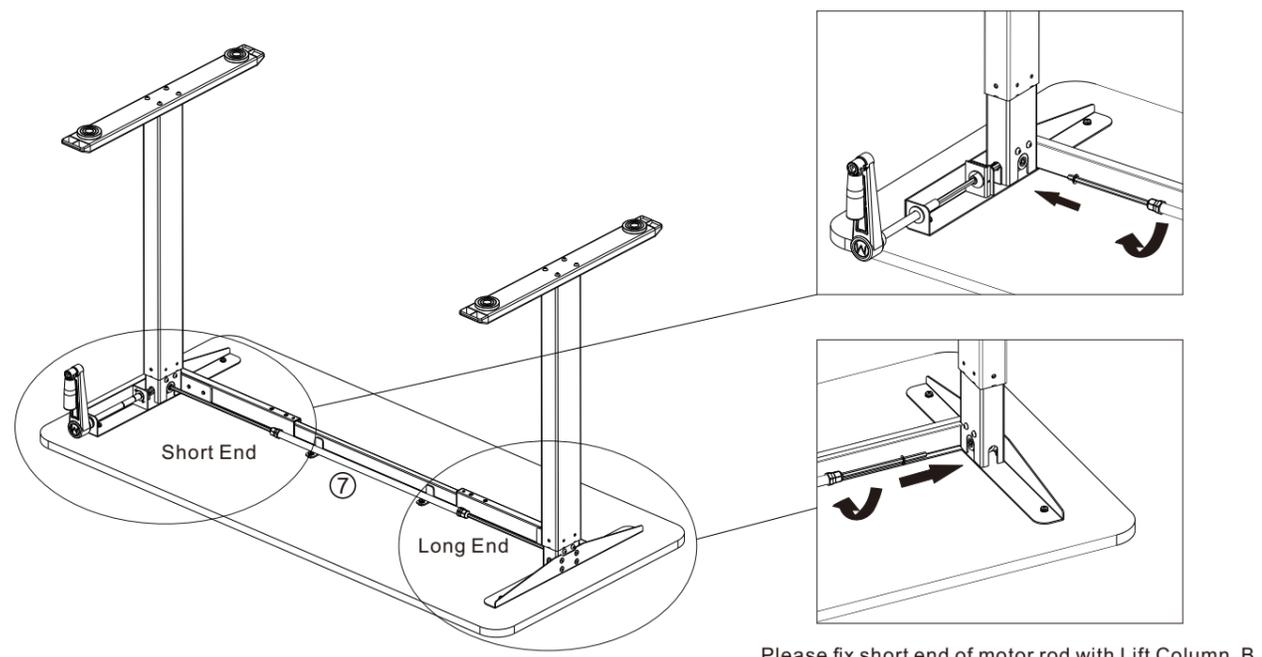
Please fix short end of motor rod with Lift Column B.
