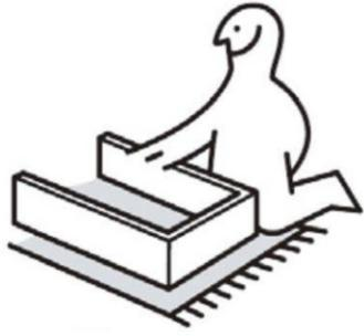
Please don't tighten the screws completely and go back later for a final tightening of all the screws after pieces are aligned with each other .
